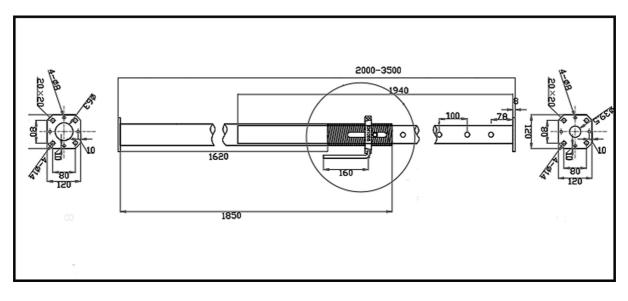
The steel prop illustrated has a nominal weight of 21.1 kg with the outer tube being 76 mm OD  $\times$  2.6 mm wall thickness and the inner tube being 63.5 mm OD  $\times$  3.1 mm wall thickness.
