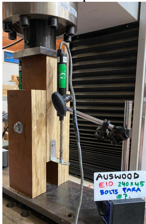
Figure A1 Typical lateral load test setup for screws/nails.
