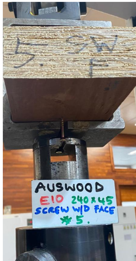
Figure A4 Typical face screw withdrawal test.
