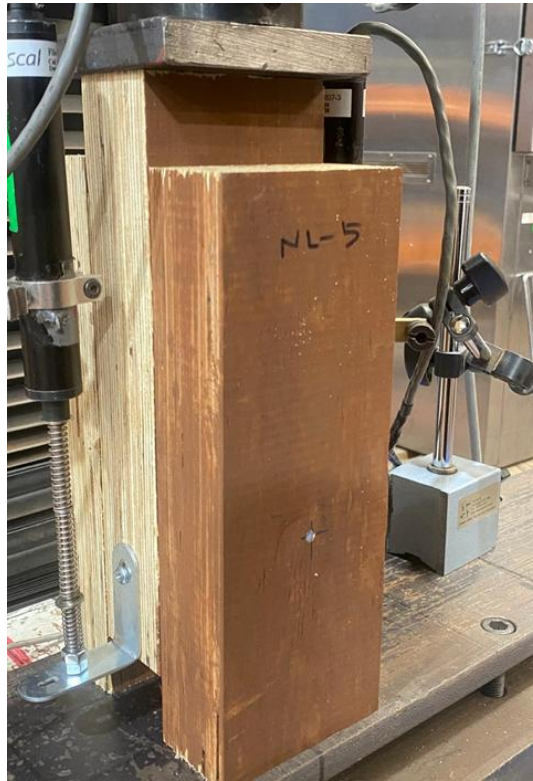
Figure A1 Typical lateral load test setup for screws/nails.
