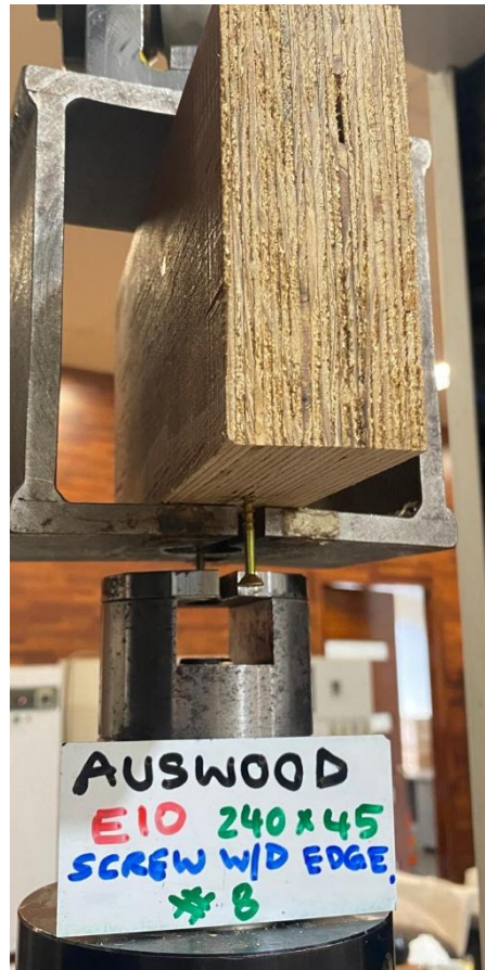
Figure A5 Typical edge screw withdrawal test.
