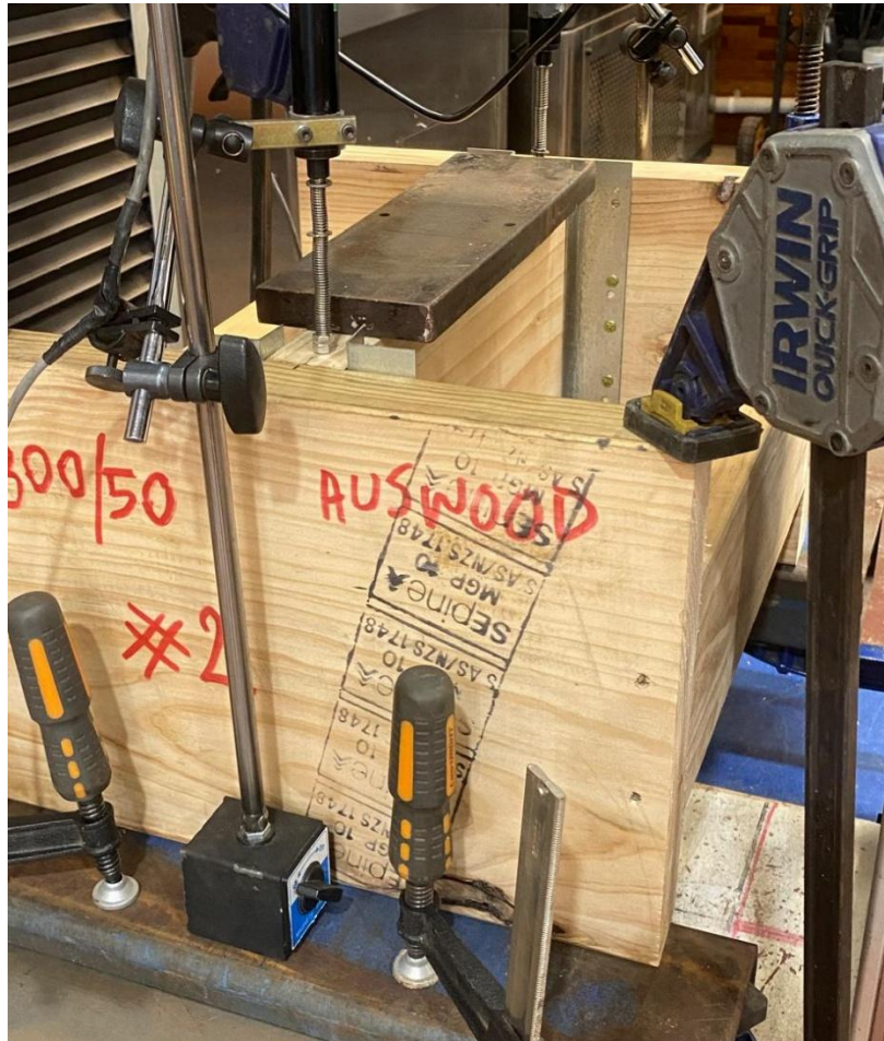
Figure 3 Joist Hanger typical test setup
